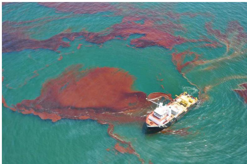
**Figure 3** Oil spill detection using optical remote sensing data. Brown color indicates oil spill [15].
