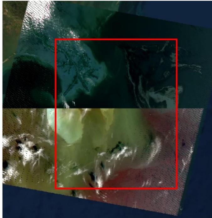
**Figure 5** Oil spill detection using the Swipe tool in ArcGIS.
