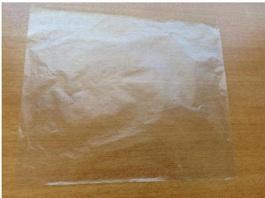
**Figure 7** Soft film made of Chitin nanofibrils (courtesy: [52]).
