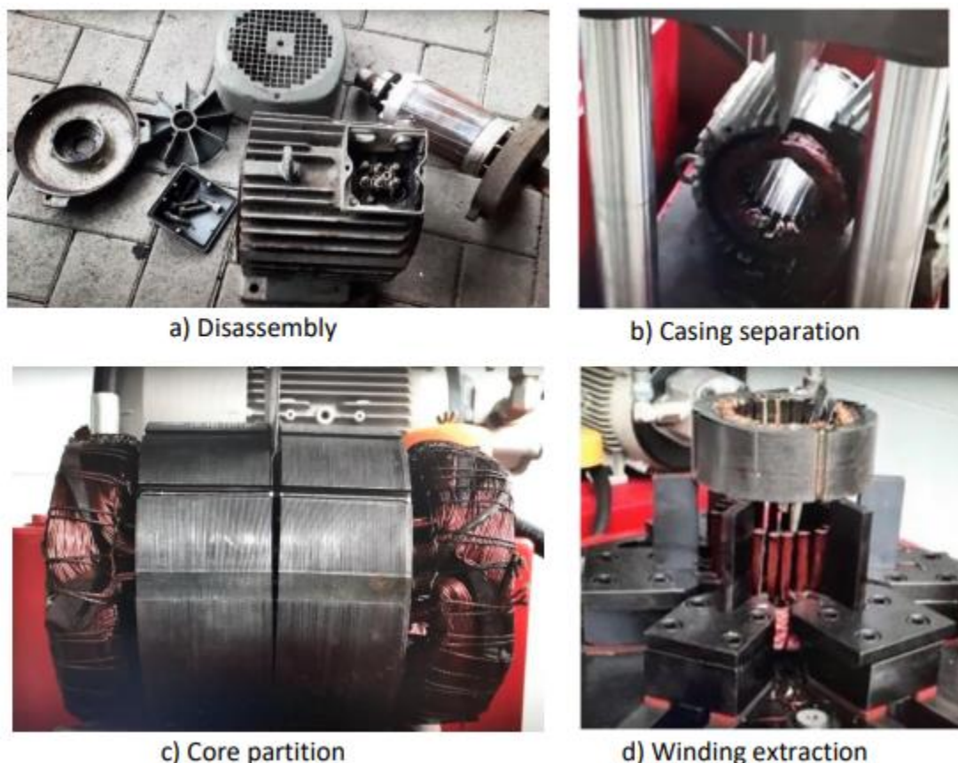
Figure 2 The disassembly process of the stator of the motor for metal recycling. (courtesy of Bronneberg, recycling machines and services, https://www.bronneberg.es ) [14].
