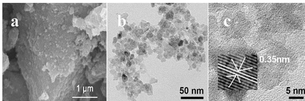
**Figure 3** The (a) SEM, (b) TEM, and (c) HRTEM images of TiO<sub>2</sub>-cellulase.
