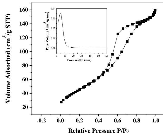
**Figure 2** The N<sub>2</sub> adsorption/desorption isotherms and the pore size distribution curves (inset) of TiO<sub>2</sub>-cellulase.
