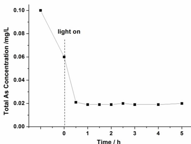
**Figure 5** The effect of reaction time on the total As concentration in aqueous dispersions (catalysts = 2.5 mg).
