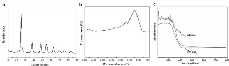
**Figure 1** (a) The XRD pattern of TiO<sub>2</sub>-cellulase. (b) The FT-IR spectrum of TiO<sub>2</sub>-cellulase. (c) The UV-Vis diffuse reflectance spectra of TiO<sub>2</sub>-cellulase and P25 TiO<sub>2</sub>.
