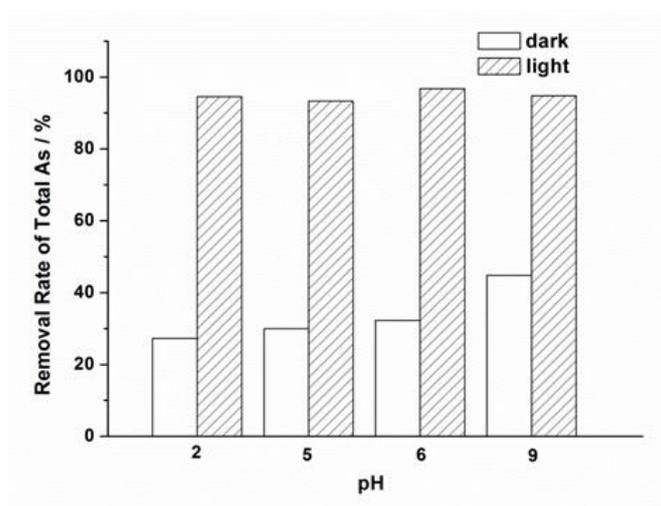
**Figure 6** Effect of pH on total As concentrations in aqueous dispersions (catalysts = 2.5 mg).
