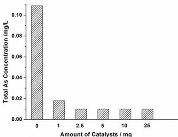
**Figure 4** The effect of the amount of catalyst on the total As concentration.
