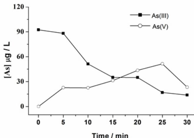
**Figure 7** Changes in the concentration of As(III) and As(V) under visible light.
