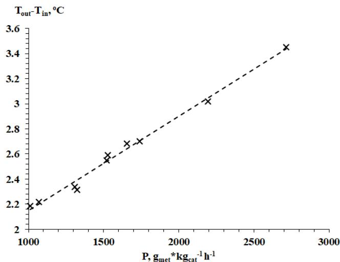
**Figure 3** Correlation of the overheating of the catalyst bed with the productivity of the catalyst during methanol synthesis.
