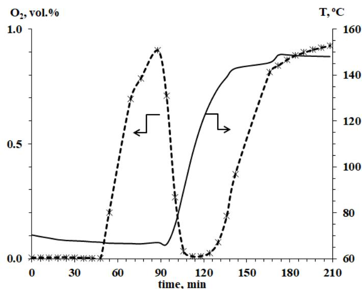
**Figure 4** Dynamics of the oxygen content at the outlet during the oxidation of the catalyst subjected to sintering conditions at 334°C.
