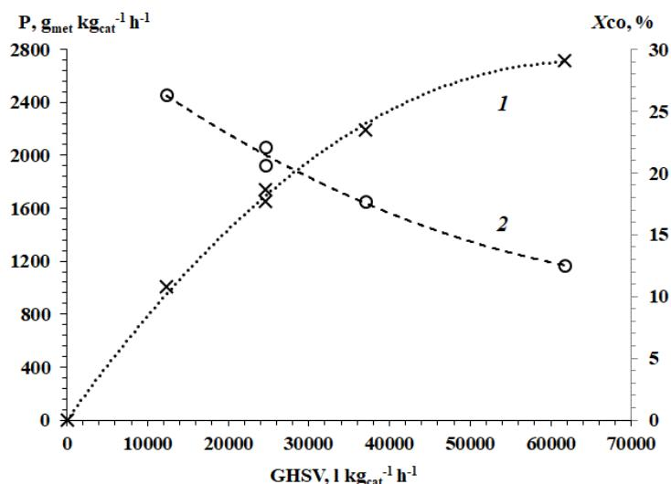
**Figure 2** Dependence of the productivity of the catalyst (1) and the conversion of CO (2) during the synthesis of methanol on the space velocity.
