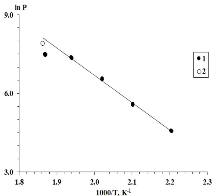
**Figure 5** Arrhenius dependence of methanol synthesis productivity. Data for GHSV: 1 – 25,000 l kg<sub>cat</sub><sup>-1</sup> h<sup>-1</sup>, 2 – 61,700 l kg<sub>cat</sub><sup>-1</sup> h<sup>-1</sup>.
