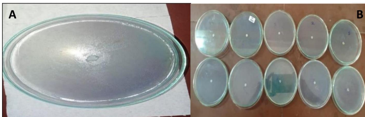
Figure 3 Test of antibacterial activity using disc diffusion assay (quantity per disc -10 \mu ) A) for R8D, B) for all synthesized 5-aryl-[1,2,4]triazolidine-3-thiones.
