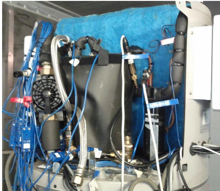
Figure 4 Test unit with insulation jacket around compressor and two filter sheets on the evaporator.
