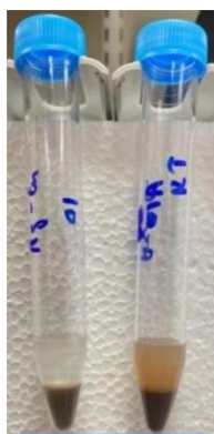
Figure 6 Synthesis of Ag- and Cu-MOBs in the same vessel. AgCysNPs and CuHARS were self-assembled in the same synthesis vessels (flasks), as described in Methods. Materials were then harvested and centrifuged in 15 ml tubes as described in Methods and resuspended in 1.5 ml of sterile water. Synthesis of materials in Tube on left was carried out at 37°C, and tube on right at 25°C. Synthesis conditions were 3 + 1 + 3 for Ag:Cu:Cystine as described in Methods. Blue scale bar at bottom of figure = 7.25 cm.
