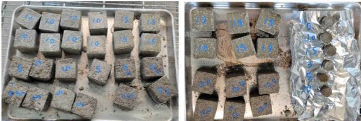
Figure 1 Preparation of cube and cylinder samples.
