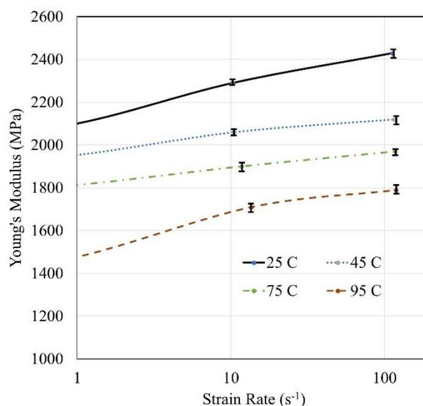
**Figure 6** Young's modulus against strain rate at four different temperatures.
