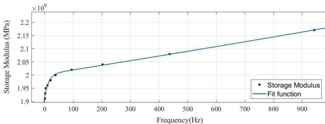
**Figure 4** Comparison of exponential fit function with storage modulus from DMA.
