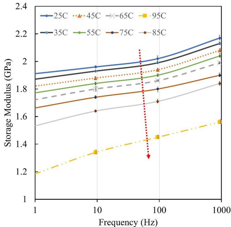
**Figure 3** Storage modulus of ABS from frequency and temperature scan using DMA.
