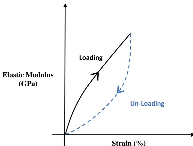
**Figure 1** Schematic of loading and unloading curves of thermoplastic polymers under sinusoidal loading.
