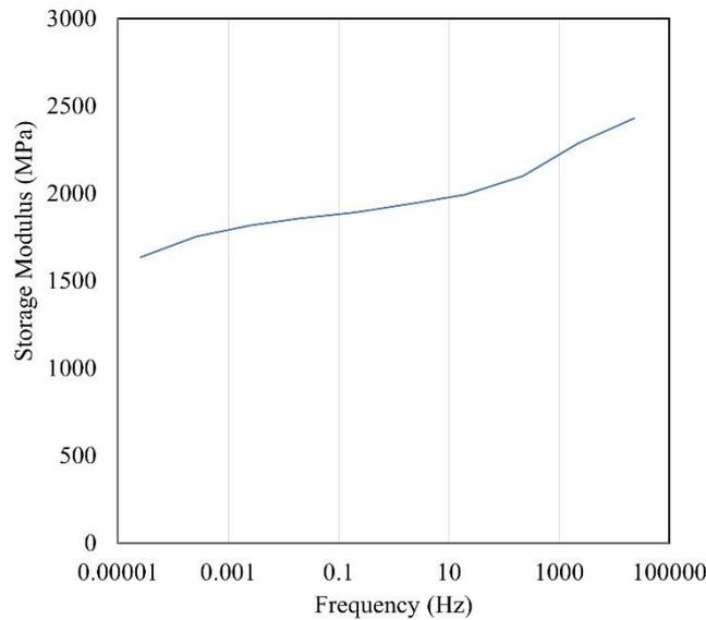
**Figure 5** Extrapolated master curve at reference temperature of 25°C using TTS and proposed fit function.
