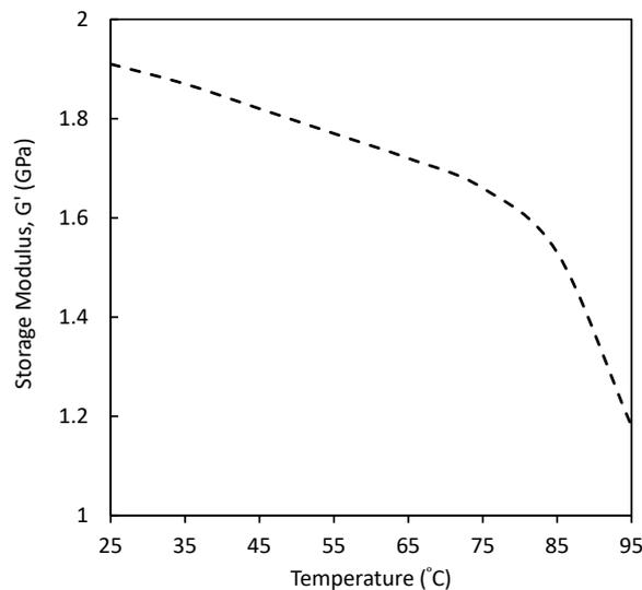
**Figure 2** Storage modulus of ABS at 1 Hz.
