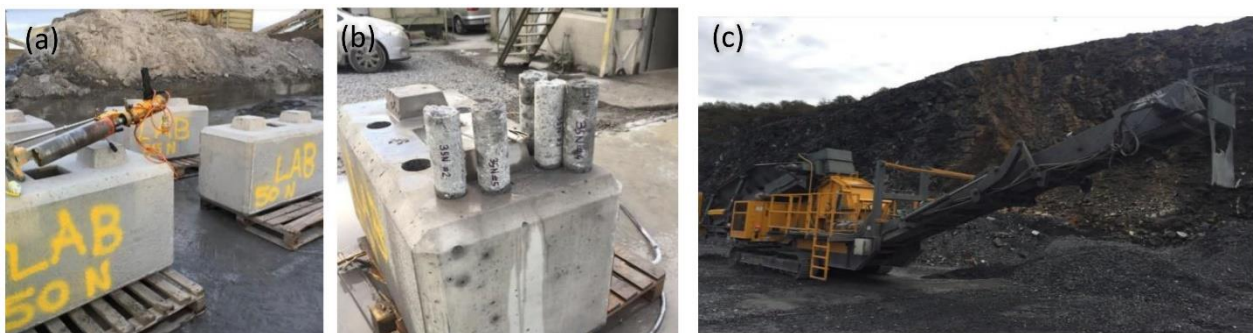
Figure 10 a) Kelly blocks, (b) Concrete cores (c) Aggregate crushing machine.
