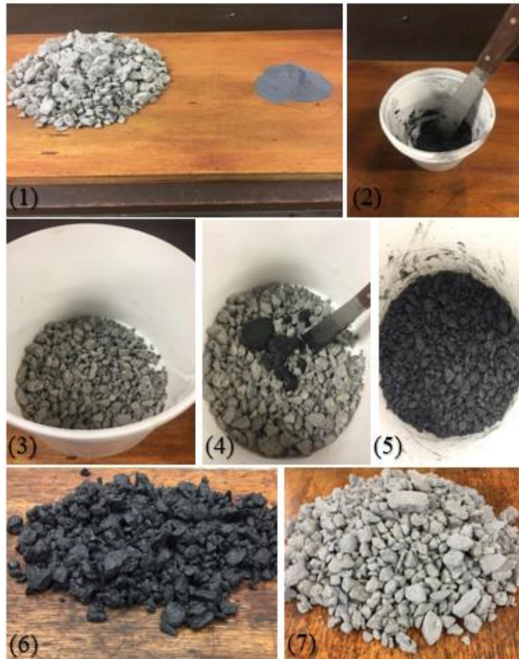
Figure 14 The steps of coating recycled aggregates with silica fume (1) dried aggregates, (2) preparing SF, (3, 4, 5) coating RCA with SF, (6) leaving the coated RCA to dry, (7) final product.
