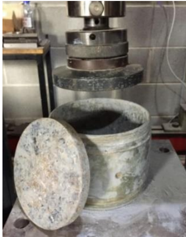
Figure 11 California bearing ratio (CBR) testing apparatus.
