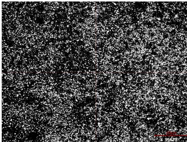
Figure 15 Surface of WC–8wt.%Co–30wt.%(B 4 C–30wt.%TiB 2 ) alloy obtained by HTS.
