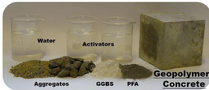
Figure 4 Typical pictorial representation of application of Geopolymer as a civil Engineering material. Source [25].
