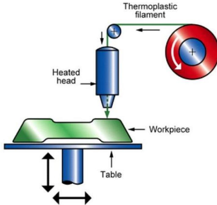
**Figure 11** Schematic of extrusion base AM technology [34].
