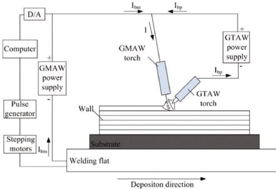
**Figure 20** Schematic diagram of double electrode GMAW-based AM [67].
