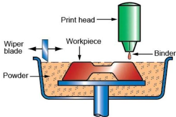
**Figure 9** Schematic of binder jetting [34].
