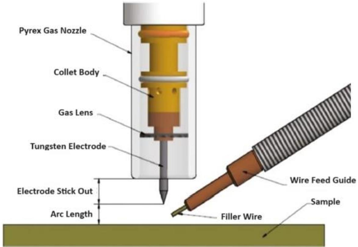
**Figure 21** Schematic of GTAW [69].
