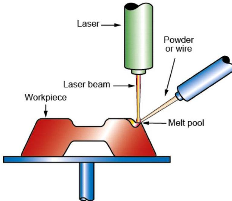
**Figure 15** Schematic of the directed energy deposition process [34].
