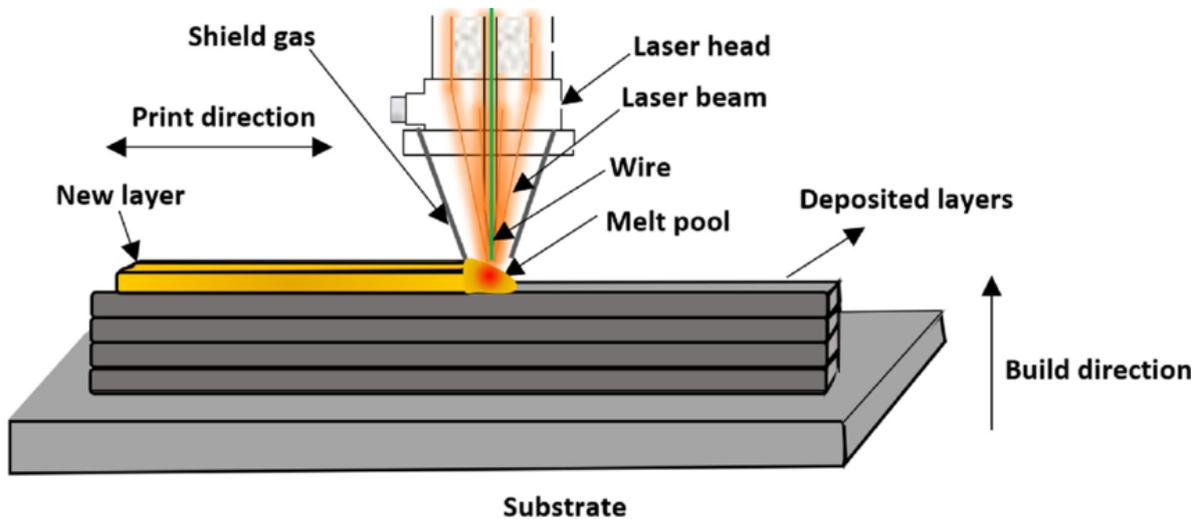
**Figure 4** Workflow Diagram of Metal Additive Manufacturing [7].
