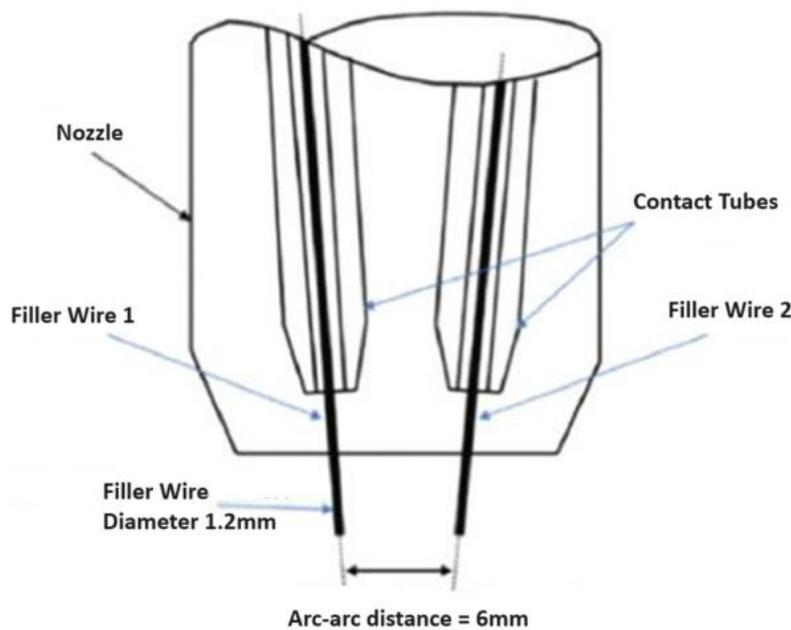
**Figure 19** Schematic of tin wire WAAM process [66].
