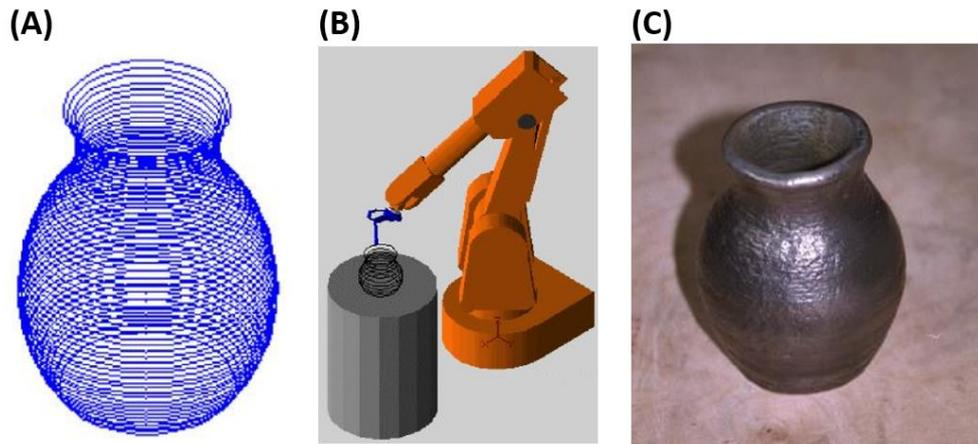
**Figure 1** Main steps of AM: (A) the object is sliced into different layers, (B) a manipulator such as a robot or machine is programmed to trace out each layer, and (C) a heat source is used to build the intended object [3].
