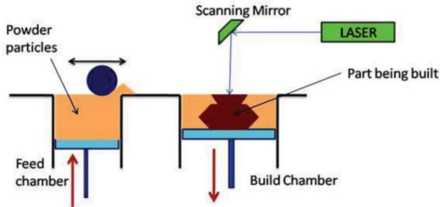
**Figure 6** Schematic of SLS Process [23].
