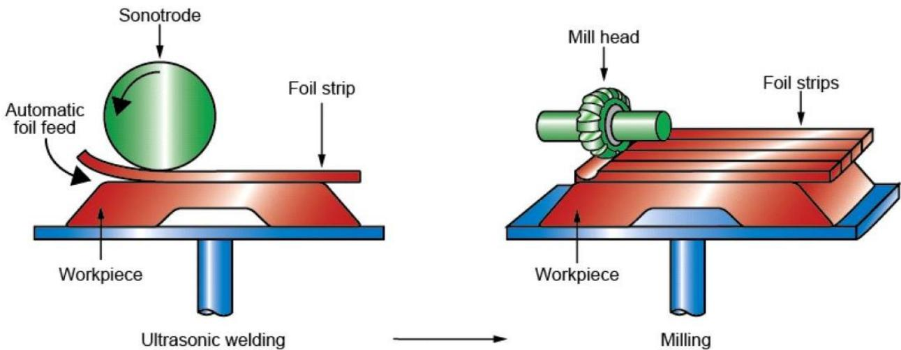
Figure 13 Sheet Lamination AM by UAM technology [34].
