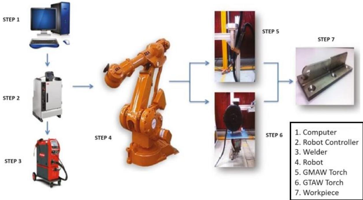
**Figure 18** Schematic of WAAM system [64].
