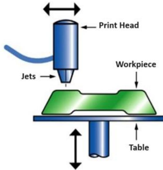
**Figure 10** Schematic of Material jetting AM [34].
