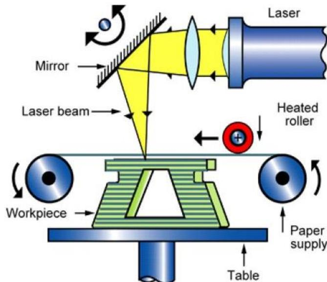
Figure 14 Sheet lamination AM by LOM technology [34].
