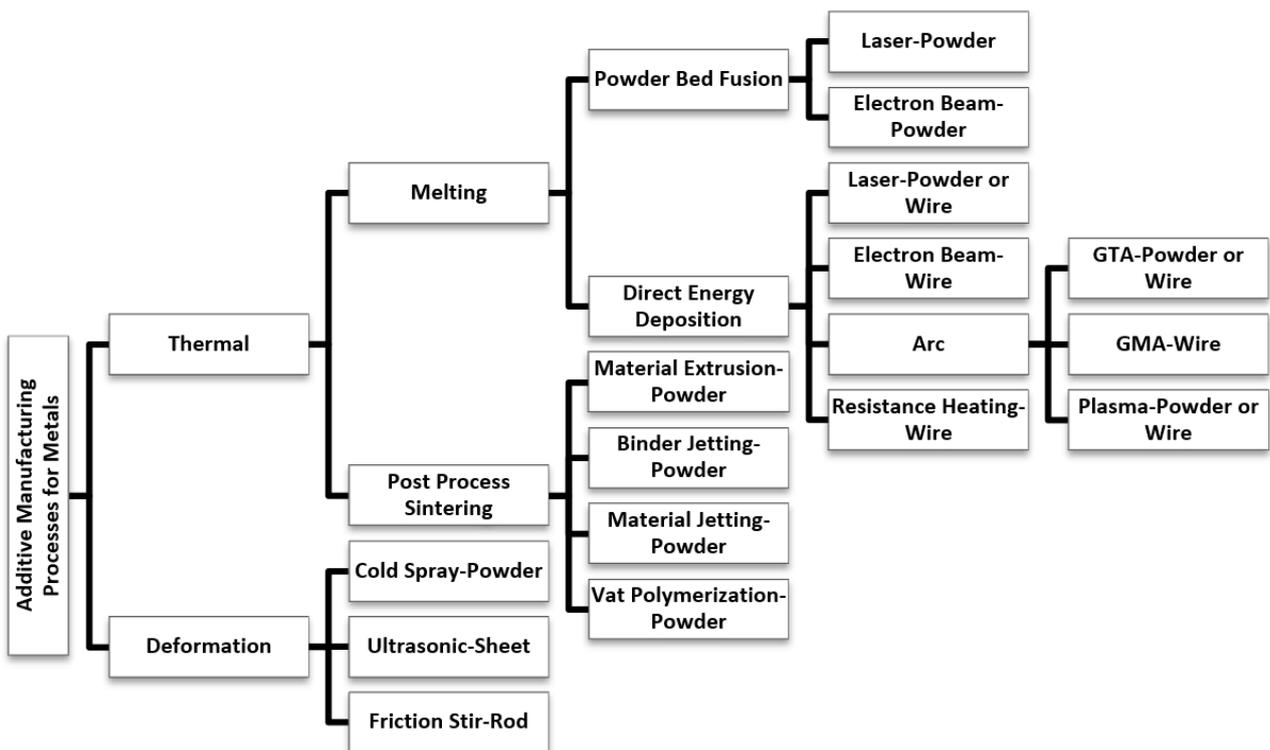
**Figure 2** Graphical representation of AM processes applicable to metals [4].
