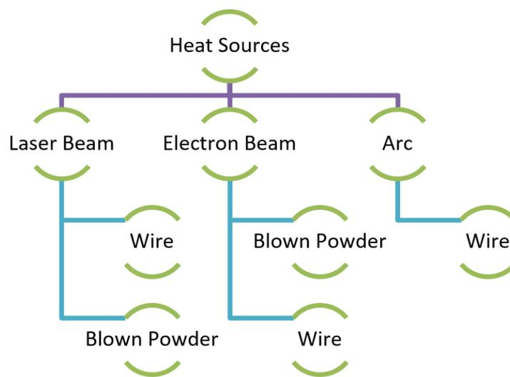
**Figure 17** Directed Energy AM techniques based on heat source and feedstock [3].
