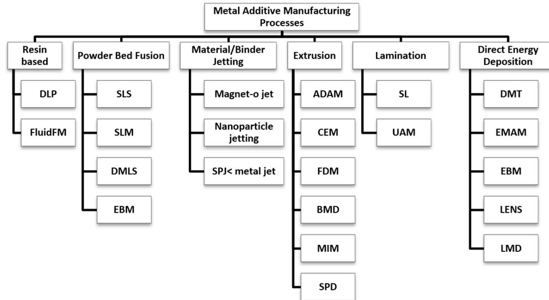
**Figure 5** Metal Additive Manufacturing Technologies<sup>1</sup> [6].
