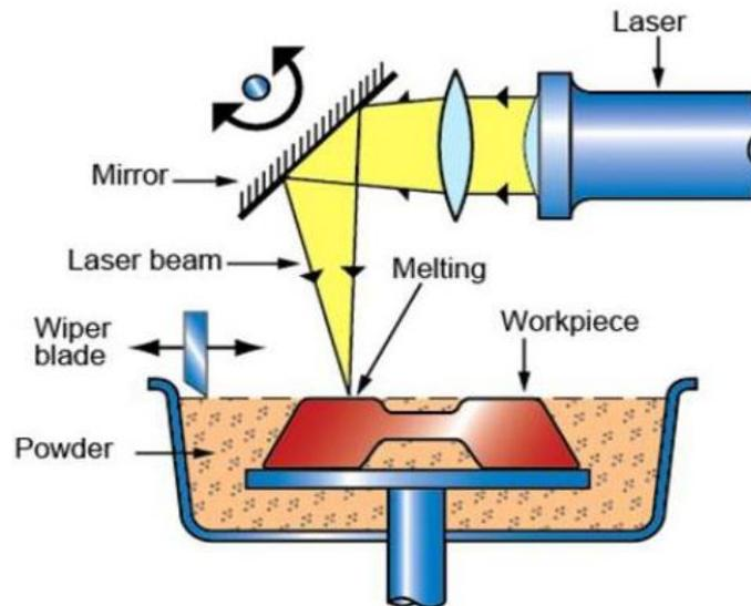
**Figure 7** Selective Laser Melting [25].
