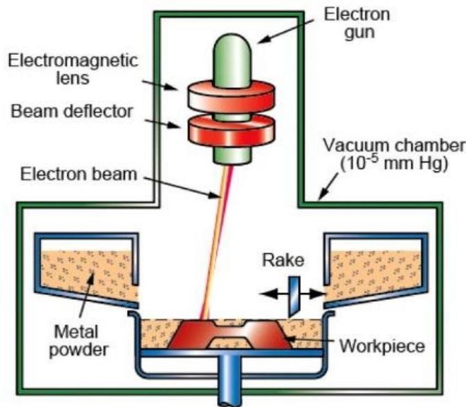
Figure 8 AM based on Electron Beam Melting [31].
