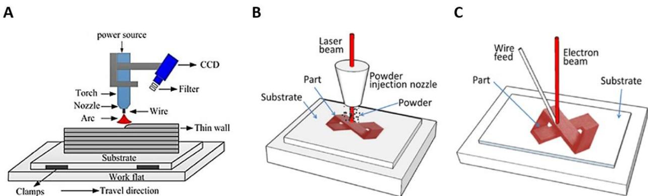
**Figure 16** Schematic of direct energy deposition by using laser beam and electron beam, respectively (A) DED-GMA [47]; (B) DED-L; (C) DED-EB [48].
