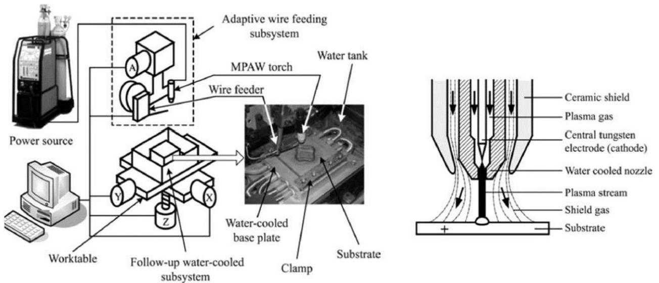
**Figure 22** Schematic of PAW based AM [63].
