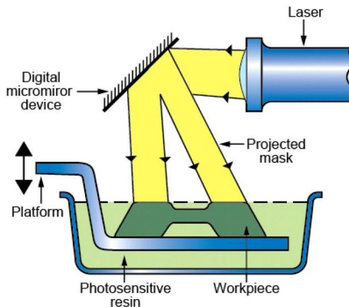
**Figure 12** Schematic of the metal resin process [43].
