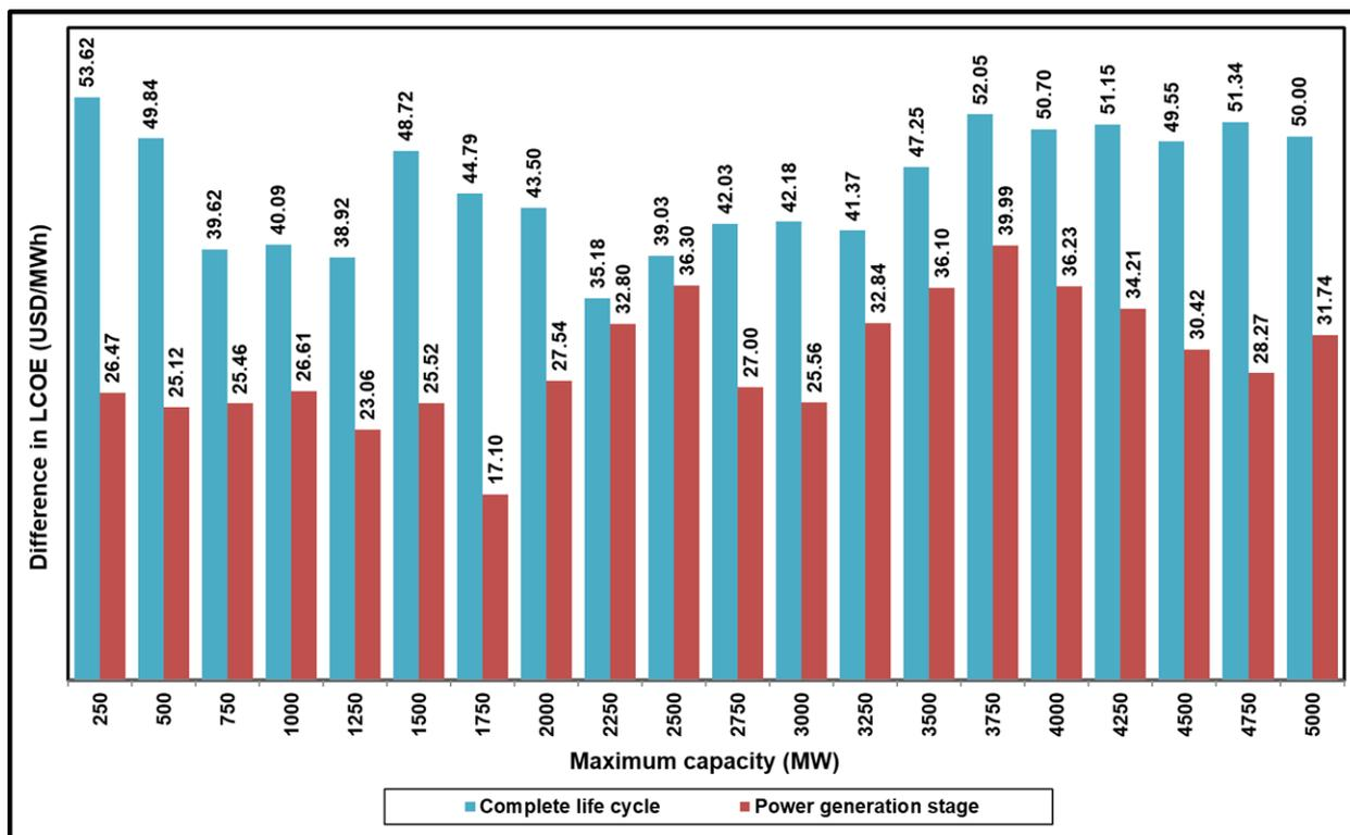
**Figure 7** Incremental increase in LCOE due to the retrofitting CCS technology on CBPG.
